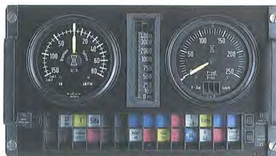
MODULAR DRIVER'S CONSOLE INDICATOR (MFA 8)
