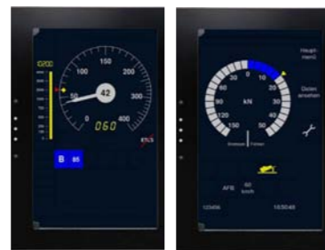
DEUTA Terminal Application for PZB Hardware concept with two DEUTA ARM terminals
